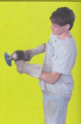
Lane Spiker uses the buffer to get some rust off a piece of metal.
