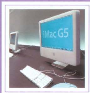
The desktop CPU of the new iMac is contained within a monitor just 2.875 inches thick.
