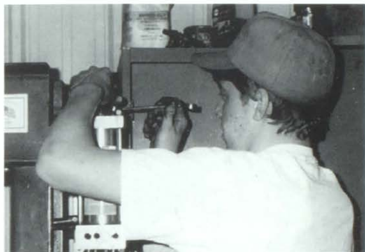
Robert Robinson is tightening a bolt on the cylinder of the bearing press in Industrial Arts. Photo by Keith Hinds.
